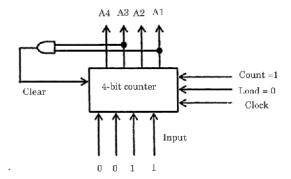
Assume that the counter and gate delays are negligible. If the counter starts at 0, then it cycles through the following sequence
