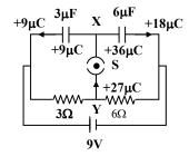
Initial charge distribution (when switch S is open)
