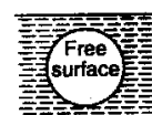
Air bubble in a liquid which also consists of only one free surface
