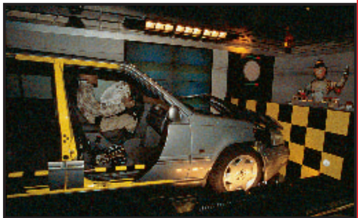
A test measures the speed at which an air bag deploys.
