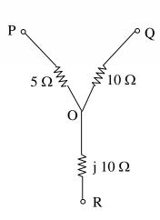
In the delta equivalent of the above star connected circuit,  $Z_{QR}$  is equal to
