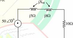
The power absorbed by the network excited by a  $50 \angle 0^0$  sinusoidal source is 168 W. The value of the mutual inductive reactance  $jX_M$  should be
