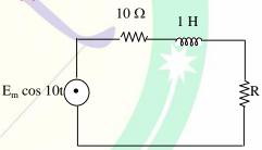
In the above circuit, the value of the load resistance R to absorb the maximum power is
