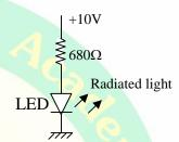
The Light Emitting Diode (LED), shown in the above figure has a voltage drop of 2V. The current flowing through LED is
