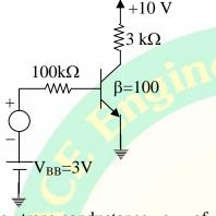
The trans-conductance  $g_m$  of the transistor used in the CE amplifier shown in the above circuit, operating at room temperature is
