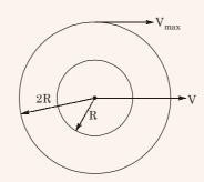
$$\begin{split} I &= & \frac{m \bigg[ \big( 2R \big)^2 - R^2 \bigg]}{2} = \frac{3}{2} m R^2 \\ V_{max} &= & 2 \omega R \\ V_{min} &= & 0 \\ V &= & \frac{V_{max} + V_{min}}{2} = \omega R \end{split}$$
