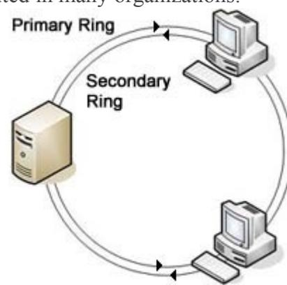
**FDDI (Fiber-Distributed Data Interface)** is a standard for data transmission on fiber optic lines in a local area network that can extend in range up to 200 km (124 miles). The FDDI protocol is based on the token ring protocol. In addition to being large geographically, an FDDI local area network can support thousands of users.
