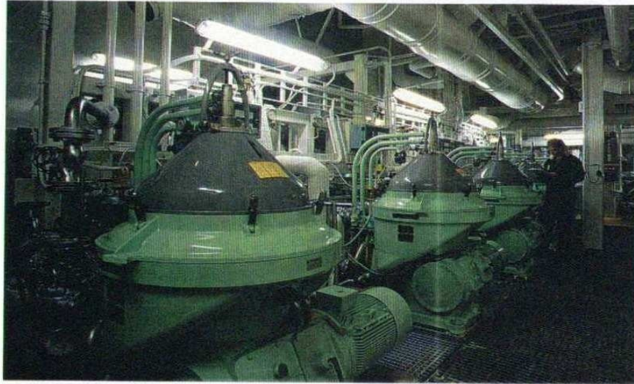
(Above) Fuel-oil separators are set in a separate machinery space adjacent to the main engine room.
