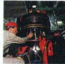
(Above) Fuel-oil separators are set in a separate machinery space adjacent to the main engine room.
