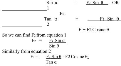
**B)** Triangle method: Now consider a force F, which is resolved into components F1 and F2. The force F makes an angle  $\alpha$  with force F<sub>1</sub> and force F<sub>2</sub> makes an angle  $\theta$  with component F<sub>1</sub>, so we can make a triangle with some suitable scale as shown in fig.
