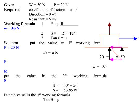
$Tan \ \theta = 0.4$   $\theta = 21.801^{\circ}$  **Result Co efficient of friction** =  $\mu = 0.4$  **Direction** =  $\theta = 21.801^{\circ}$ **Resultant** = S = 53.85 N
