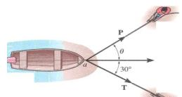
13. A disabled automobile is pulled by means of two ropes as shown. Knowing that the tension in the rope P is 500 lb, determine the tension in rope T and the value of so that the resultant force exerted is as 800 lb force directed along the axis of the automobile
