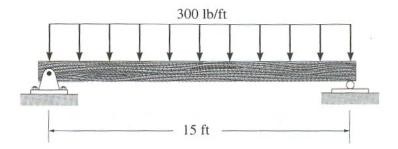
14 Find the reaction at the points as shown in diagram
