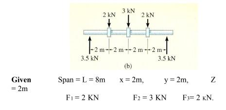
Shear force and moment diagram Required Solution Take moment about "A" also consider the upward force clock moment and wise is positive  $\sum M_A = 0$  $R_E(L) - F3(x + y + z) - F_2(x + y) - F_1(x) + R_A$ (0) = 0. $R_E(8) - 2(6) - 3(4) - 2(2) + 0 = 0$  $R_E = 3.5 \text{ KN}$ Now for RA we can calculate by  $\Sigma F = 0$  $R_{A} - F_{1} - F_{2} - F_{3} + R_{E} = 0$  $R_A - 2 - 3 - 2 + 3.5 = 0$
