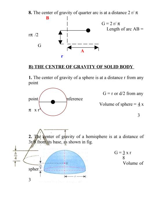
**3.** The gravity of right circular solid cone is at a distance h/4 from its base, measured along the vertical axis
