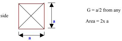
4. The center of gravity of a parallelogram is at a point, where its diagonals meet each other. It is also a mid point of the length as well as the height of the parallelogram as shown in fig
