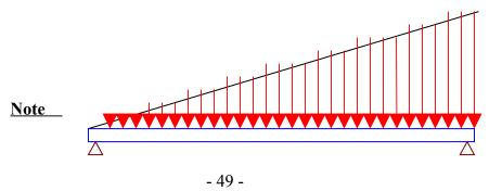
Any beam may be point, uniformly distributed and uniformly varying load
