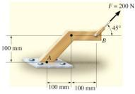
Given F=200N  $\theta = 45^{\circ}$ Required  $M_A =?$ Solution Resolve the force into components  $F_1$  am  $F_2$   $F_1 = F \cos \theta$   $F_1 = 200 \operatorname{cosine} 45^{\circ}$   $F_1 = 141.42N.$   $F_2 = F \sin \theta$   $F_2 = 200 \sin 45^{\circ}$   $F_2 = 2.468N.$ We know that  $M_A = 0$
