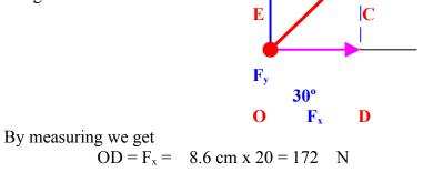
$OE = Fy = 5 \text{ cm } x \ 20 = 100 \text{ N}$ **Result:**  $F_x = 173.20 \text{ N}$  $F_{v} = 100 N$ B) <u>Analytically</u> We know that  $F_x = F \text{ cosine } \theta$ = 200 cosine 30 $F_x = 173.20 \text{ N}$ We also know that  $F_v = F \sin \theta = 200 \sin 30$  $F_{v} = 100$ Ν  $F_v = 100 N$ **Result:**  $F_x = 173.20 N$
