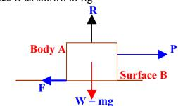
A little concentration will show that the body A presses the surface B downward equal to weight of the body and in reaction surface B lift the body in upward direction of the same magnitude but in opposite direction therefore the body in equilibrium this upward reaction is termed as normal reaction and it is denoted by R or N.
