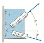
13. The two structural member one in tension and other in compression, exerts on point O, determine the resultant and angle  $\theta$
