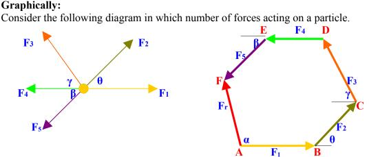
Starting from A the five vectors are plotted in turns as shown in fig by placing the tail end of each vector at the tip end of the preceding one. The arrow from A to the tip of the last vector represents the resultant of the vectors with suitable scale. In this polygon the side AF represents the resultant of the given components and  $\alpha$  shows the direction. By measurement of AF will give the resultant and  $\alpha$  give direction of given scale
