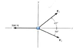
12. Determine the magnitude and direction of  $F_1$  and  $F_2$  so that the partial is in equilibrium
