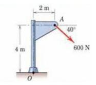
13. A force F of magnitude 400 N is applied. Determine the magnitude of moment about point  $\Omega$
