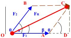
We can also determine the components of force F by analytically as we know that direction of the resultant vector can be determined by
