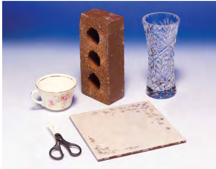
Figure 1. Common objects that are made of ceramic materials: scissors, a china tea cup, a building brick, a floor tile, and a glass vase.
