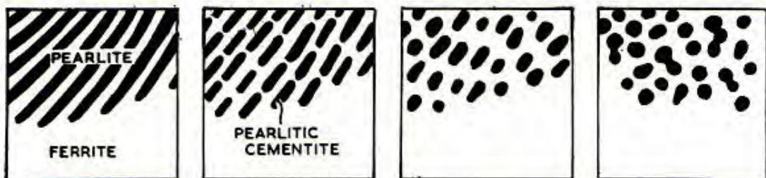
Figure 3. The Spheroidisation of Pearlitic Cementite.
