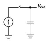
If the switch is closed at t = 0, which of the following plots depicts correctly the output voltage of the circuit as a function of time?
