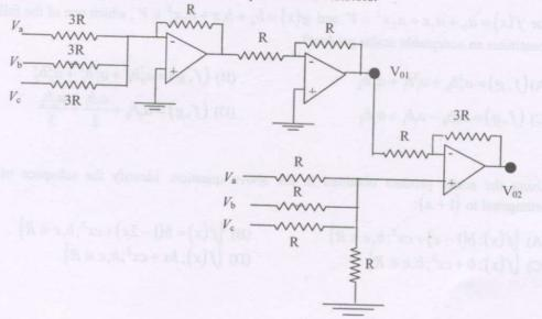
Q.82 The output voltage at the end of second operational amplifier V<sub>01</sub> is
