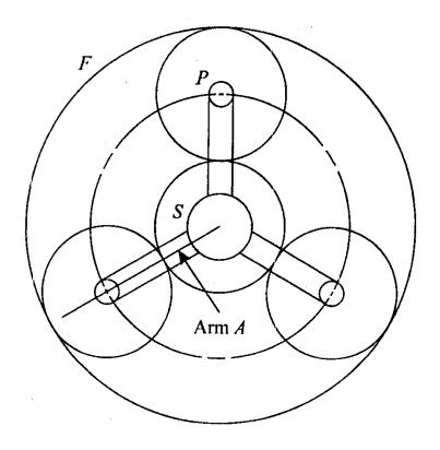
In the geartrain shown in the figure, the sun gear S rotates at 500 rpm and the planet carrier A rotates at 100 rpm in the same direction. Determine the number of teeth on each gear and the speed of planet gear P if the diametral pitch of all the gears is 3 teeth/cm and the diameter of the fixed gear F is to be as close to 25 cm as possible.
