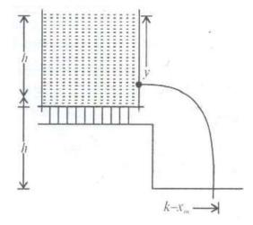
A tank is filled up to a height h with a liquid and is placed on a plateform of height h from the ground. To get maximum range  $x_m$ , a small hole is punched at a distance y from the free surface of the liquid. Then
