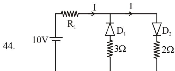
Diode  $D_1$  is reversed biased. Then no current will flow through that link.
