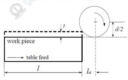
If t is the depth of cut and d is the diameter of the milling cutter, then the length of approach  $(l_a)$  is expressed as
