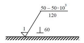
The waviness height (in micrometer) of the surface is
