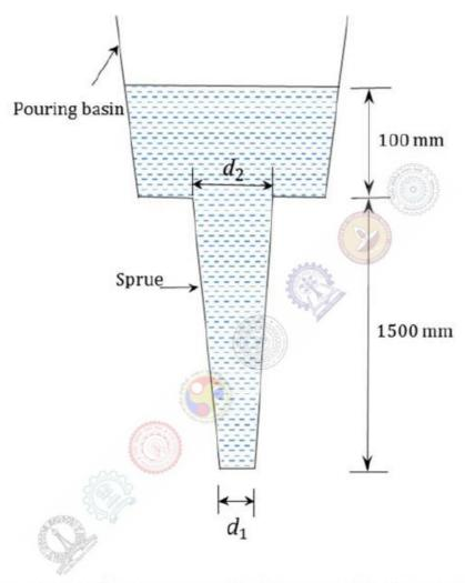
Considering the cross-section of the sprue is circular, the ratio  $d_1:d_2$  to avoid aspiration is
