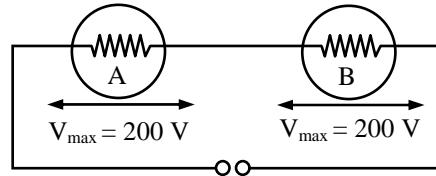
$$V_1 = \frac{V \times R_1}{R_1 + R_2} = 200$$
