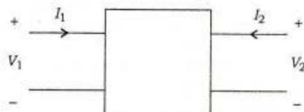
$$V_1 = 60I_1 + 20I_2 \quad \text{and} \quad V_2 = 20I_1 + 40I_2$$
