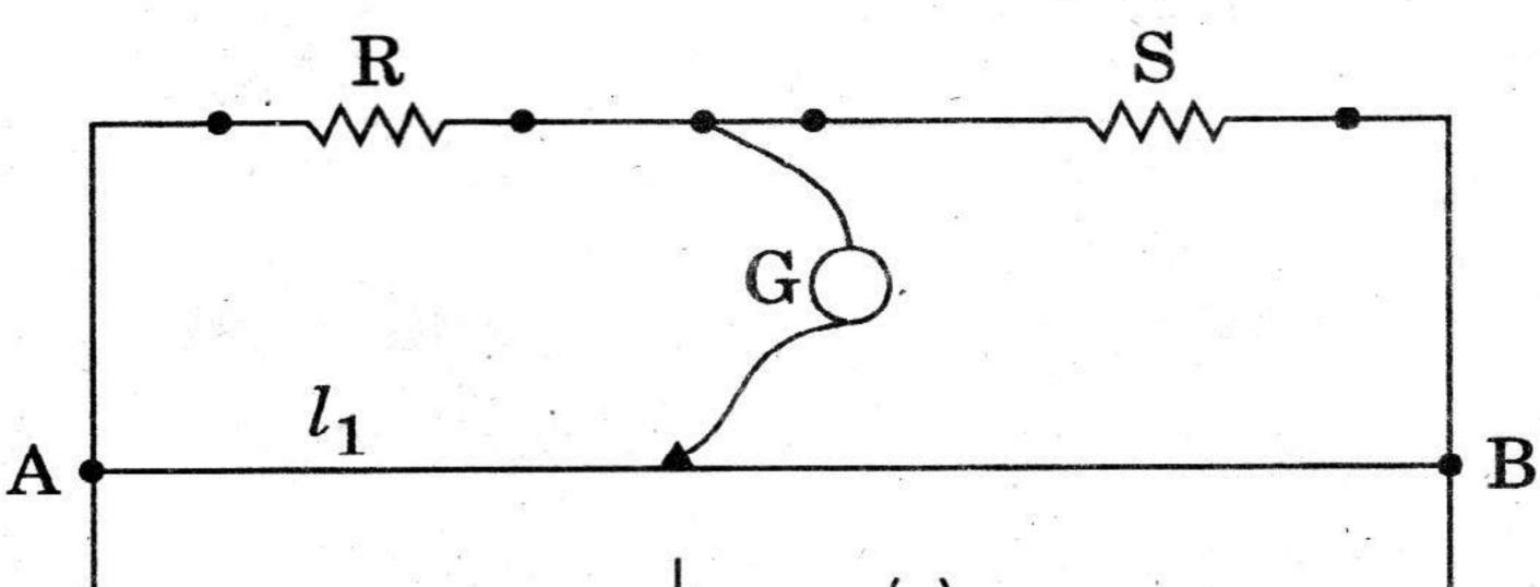
An unknown resistance X is now connected in parallel to the resistance S and the balance point is found at a distance  $l_2$ . Obtain a formula for X in terms of  $l_1$ ,  $l_2$  and S.
