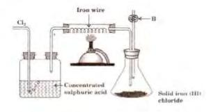
(a) The diagram given below is to prepare iron(III) chloride in the laboratory:
