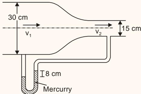
When the water flows, the differential manometer shows a deflection of 8cm of mercury (Hg). The values of specific gravity of mercury and water are 13.6 and 1.0, respectively. Consider the acceleration due to gravity,  $g = 9.81 \text{ m/s}^2$ . Assuming frictionless flow, the flow rate (in  $\text{m}^3/\text{s}$ , round off to 3 decimal places) through the duct is \_\_\_\_\_.
