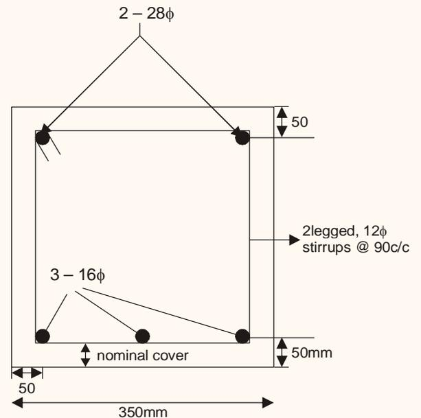
$$\therefore \text{Nominal cover} = \left(50 - \frac{16}{2} - 12\right) \text{ mm} = 30 \text{ mm}$$
