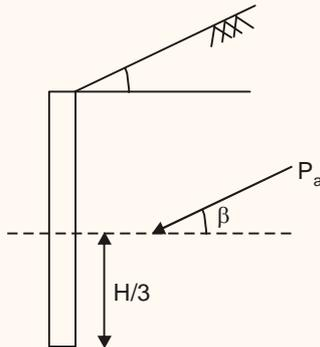
active thrust act at a height  $H/3$  from the base of the wall and at an angle equal to backfill inclination.
