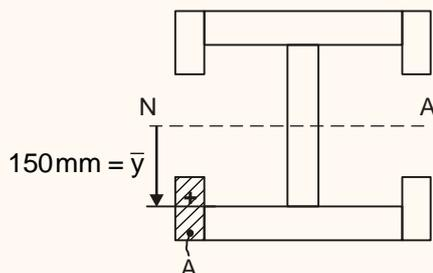
Shear force in nail at P =  $\frac{VA\bar{y}}{I} \times \text{pitch}$
