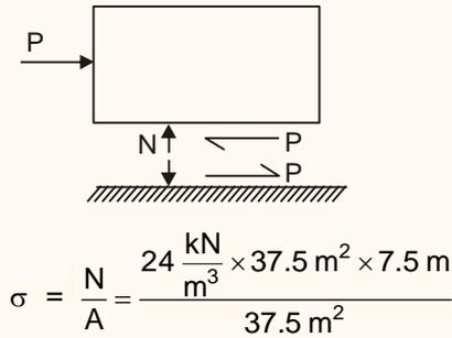
$$\sigma = \frac{N}{A} = \frac{24 \frac{\text{kN}}{\text{m}^3} \times 37.5 \text{ m}^2 \times 7.5 \text{ m}}{37.5 \text{ m}^2}$$
