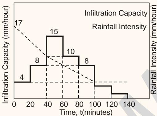
Depth of infiltration = Area of hyetograph above Horton's curve
