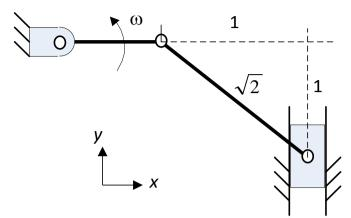
Using exact analysis, the acceleration of the slider in the *y*-direction, at the instant shown, where the crank is parallel to *x*-axis, is given by
