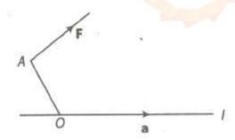
Let F be a force acting at a point A, O be any point on the given line L and a be the unit vector along the line, then moment of F about the line L is a scalar given by  $(OA \times F) * a$
