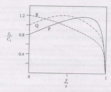
In the above figure,  $c_l$  refers to the section lift coefficient,  $C_L$  refers to the lift coefficient of the wing, y is the coordinate along the span and s is the span of the wing. A designer prefers to use a wing for which the stall begins at the root. Which of the wings will he choose?
