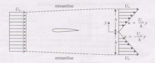
The flow of density  $\rho$  is incompressible, two dimensional and steady. The pressure is  $p_{\infty}$  over the entire surface of the control volume. The drag on the airfoil is given by,
