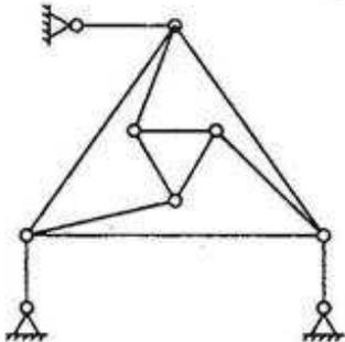
I. The truss is statically determinate
