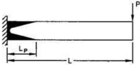
The length  $L_p$  of the plastic zone, when the maximum bending moment, equals the plastic moment  $M_p$ , given by
