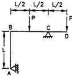
The reaction at the roller end A is given by
