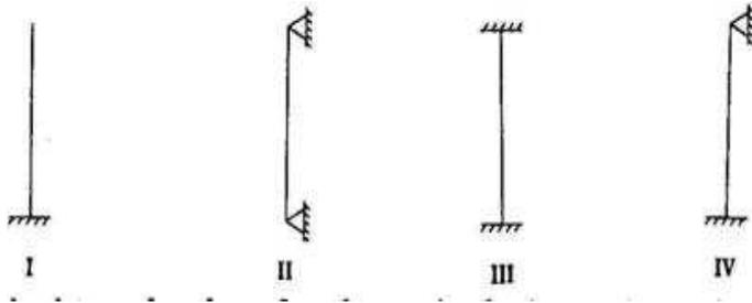
It is required to order these four beams in the increasing order of their respective first buckling loads. The correct order is given by
