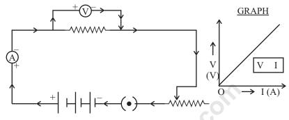
**Ohm's Law** He stated that the electric current flowing through a conductor is directly proportion at to the potential difference across its ends, provided the temperature remain constant
