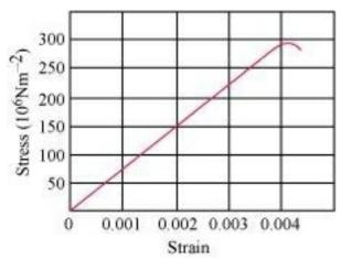
**Ans. (a)** It is clear from the given graph that the stress  $150 imes 10^6~N/m^-2$  , strain is 0.002.
