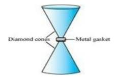
**Ans.** Diameter of the cones at the narrow ends,  $d = 0.50 \text{ mm} = 0.5 \times 10^{-3} \text{ m}$
