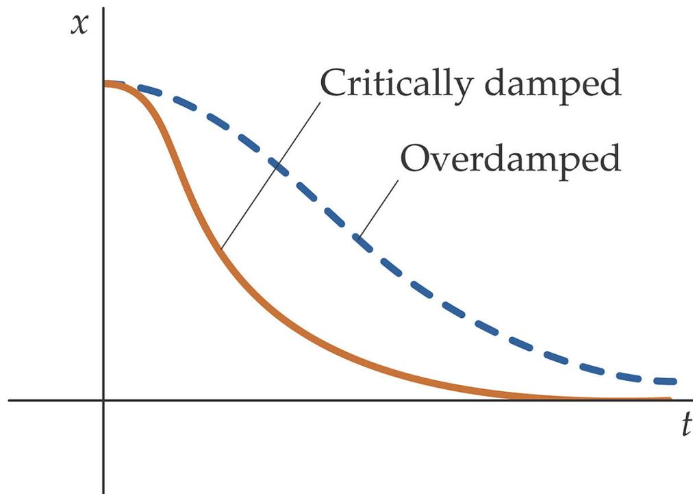
The larger the damping the more difficult it is to assign a frequency to the oscillation.
