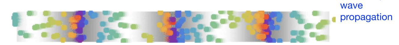
this is a sinusoidal wave so each particle is undergoing Simple Harmonic Motion
