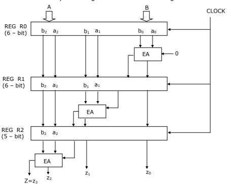
(a) For 8 clocks pulses on the CLOCK terminal and the inputs A, B as shown, obtain the output Z (sequence of 4-bit values of Z). Assume initial contents of R0, R1 and R2 as all zeros.
