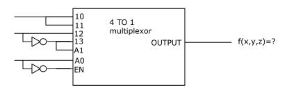
The function f(x,y,z) implemented by the above circuit is
