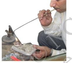
Fig. 6.11 : Goldsmith blowing through a metallic pipe
