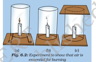
chimney [Fig. 6.2(a)]. Observe what happens to the flame. Now remove the blocks and let the chimney rest on the table [Fig. 6.2(b)]. Again observe the flame. Finally, put a glass plate over the chimney [Fig. 6.2(c)]. Watch the flame again. What happens in the three cases? Does the flame flicker off? Does it flicker and give smoke? Does it burn unaffected? Can you infer anything at all about the role played by air in the process of burning?
