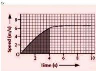
The greyed out region of the graph that is equal to 0.5 \* 4 \* 6 = 12m, stands for the distance travelled by the bike in first four kilometers.
