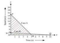
Distance travelled by each car after the application of brakes is given by the area under their respective speed-time graph
