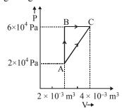
In process AB, 400 J of heat is added to the system and in process BC, 100 J of heat is added to the system. The heat absorbed by the system in the process AC will be [2015]
