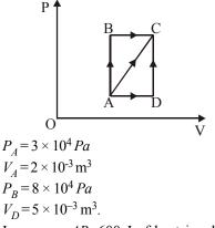
In process AB, 600 J of heat is added to the system and in process BC, 200 J of heat is added to the system. The change in internal energy of the system in process AC would be [1991] (b) 800 J
