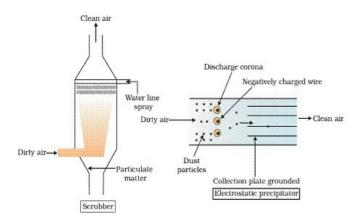
It has electrode wires that are maintained at several thousand volts to produce a corona that releases electrons. These electrons attach to dust particles giving them a net negative charge. The collecting plates are grounded and attract the charged dust particles to that clean air can pass through electrostatic precipitator.
