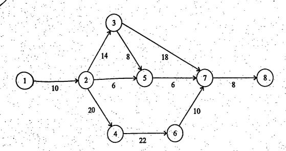
Identify the critical path in the network as shown in figure and determine the project completion time. The duration are in weeks.
