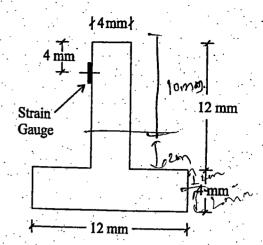
A small T-section is used in inverted position as a beam and is shown in figure over a span of 400 mm. If due to the application of forces shown, the longitudinal strain gauge at F registers a compressive strain of 1500 microstrains, determine the magnitude of P. Take E=200 GPa.
