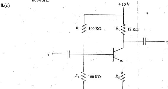
(i) Common emitter (CE) amplifier shown in the figure has voltage gain 400 when  $R_E = 0$ . Stability is brought through negative feedback by adding resistor  $R_E$ . Find the value of resistor  $R_E$  using feedback concepts so that final voltage gain is equal to 200.
