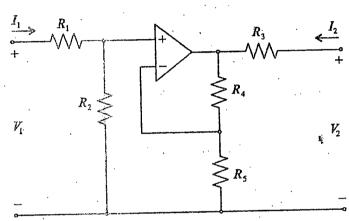
Find the z parameters of the network shown in the figure. Is the network reciprocal? If so why? Assume the operational amplifier is ideal.
