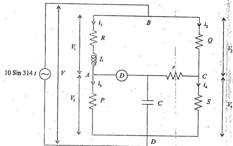
The bridge network shown in the figure measures the inductance (L) and resistance (R) if the impedance between A and B is unknown.
