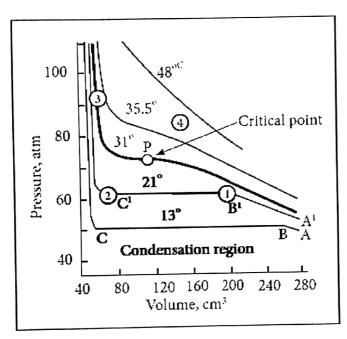
At low temperature isotherms, for example, at 13<sup>o</sup>C as the pressure increases, the volume decreases along AB and is a gas until the point B is reached.
