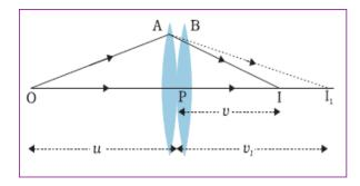
For the first lens, object is at O and image is at I<sub>1</sub>.
