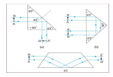
Total reflecting prisms are used in periscopes.
