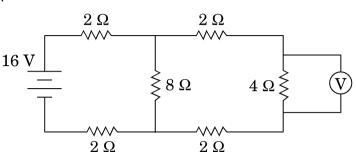
In the circuit given below, find the voltmeter reading across a 4  $\Omega$  resistor.
