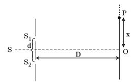
(c) In Young's double slit experiment, the slits are separated by 0.5 mm and screen is placed 1.0 m away from the slit. It is found that the 5<sup>th</sup> bright fringe is at a distance of 4.13 mm from the 2<sup>nd</sup> dark fringe. Find the wavelength of light used.
