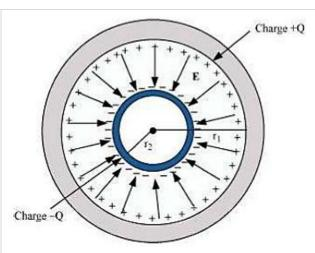
that the capacitance of a spherical capacitor is given by
