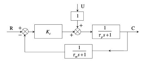
A unit step input is introduced in the set point. The value of  $K_c$  to provide a critically damped response for U=0,  $\tau_p=8$  and  $\tau_m=1$  is
