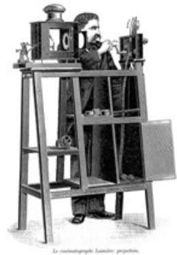
Fig1.7 (B) Cinematographe in projection mode
