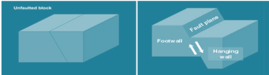
Fig. 4.24: Normal fault showing the relative downward movement of hanging wall
