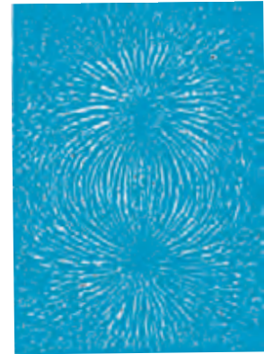
FIGURE 5.2 The arrangement of iron filings surrounding a bar magnet. The pattern mimics magnetic field lines. The pattern suggests that the bar magnet is a magnetic dipole.
