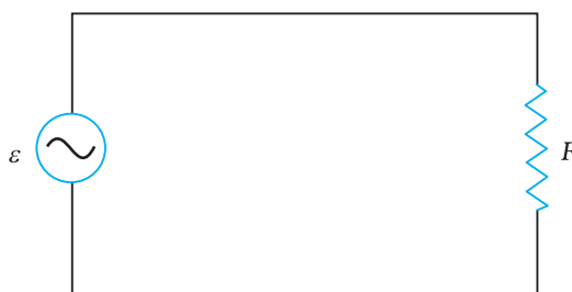
FIGURE 7.1 AC voltage applied to a resistor.
