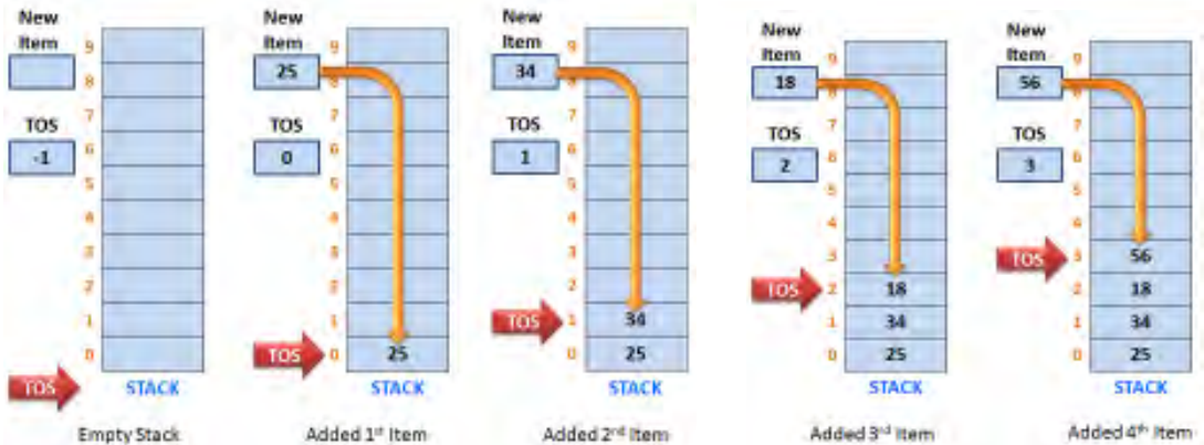
Fig. 3.5: Status of stack after a sequence of push operations
