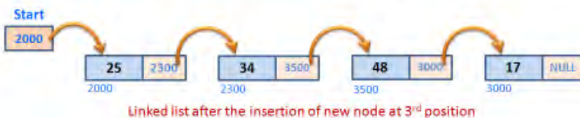
Fig. 3.18: Insertion operation in a linked list
