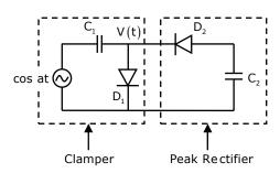
When excited by cos ( $\omega t$ ), the clamping section clamp the positive peak to 0 volts and negative peak to -2 volts. So whole  $\cos(\omega t)$  is lower by -1 volts
