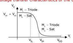
where  $V_{\text{IL}} = \frac{1}{8} \big( 3 V_{\text{DD}} + 2 V_{\text{t}} \big) = 2.125 V$  , Hence Option 'A' is approximately
