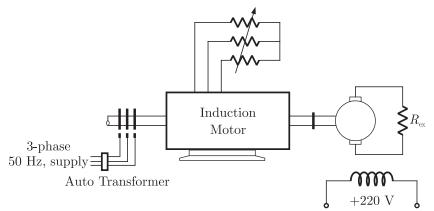
The motor is coupled to a 220 V, separately excited d.c generator feeding power to fixed resistance of 10  $\Omega$ . Two-wattmeter method is used to measure the input power to induction motor. The variable resistance is adjusted such the motor runs at 1410 rpm and the following readings were recorded  $W_1 = 1800$  W,  $W_2 = -200$  W.
