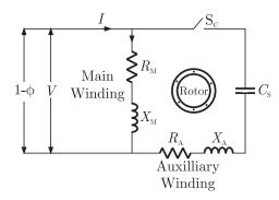
The two windings are displaced  $90^{\circ}$  in space. The direction of rotation can be changed by reversing the main winding terminals.
