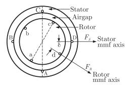
The following table gives four set of statement as regards poles and torque. Select the correct set corresponding to the mmf axes as shown in figure.
