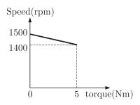
**MCQ 4.14** The armature resistance of the motor is
