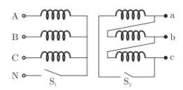
The star-delta transformer shown above is excited on the star side with balanced, 4-wire, 3-phase, sinusoidal voltage supply of rated magnitude. The transformer is under no load condition
