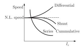
The shunt motor provides speed regulation at full load without any controller.
