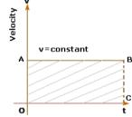
That is the area under the Velocity – time graph represents the displacement.
