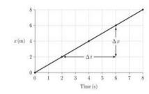
That is the slope of position time graph gives the Velocity.
