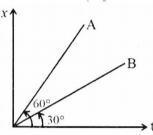
Ans: a) Body A.[The slope of position time graph gives the velocity. Higher the slope greater the velocity]
