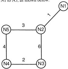
The network uses a Distance Vector Routing protocol. Once the routes have stabilized, the distance vectors at different nodes are as following.
