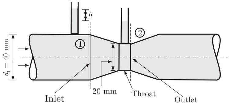
Given :  $d_2 = 20 \text{ mm} = 0.020 \text{ m}$ ,  $d_1 = 40 \text{ mm} = 0.040 \text{ m}$
