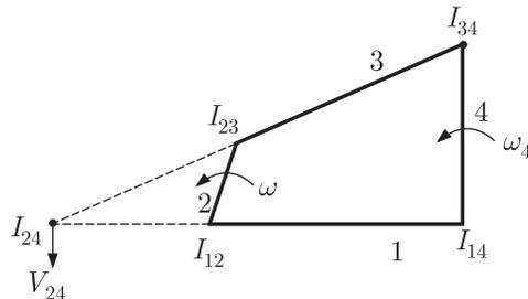
From the angular velocity ratio theorem.
