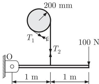
Given :  $r = 200 \text{ mm} = 0.2 \text{ m}$ ,  $\theta = 270^\circ = 270 \times \frac{\pi}{180} = \frac{3\pi}{2}$  radian,  $\mu = 0.5$
