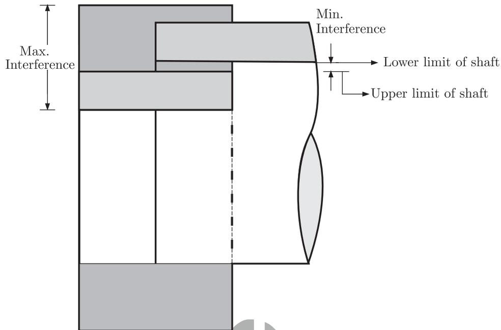
The interference is the amount by which the actual size of a shaft is larger than the actual finished size of the mating hole in an assembly.
