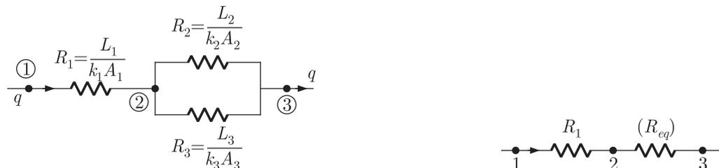
$$R_1 = \frac{L_1}{k_1 A_1} = \frac{0.5}{0.02(1 \times 1)} = 25 \text{ K/W}$$
