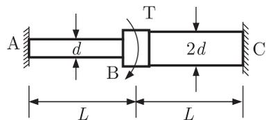
Here both the shafts  $AB$  &  $BC$  are in parallel connection.
