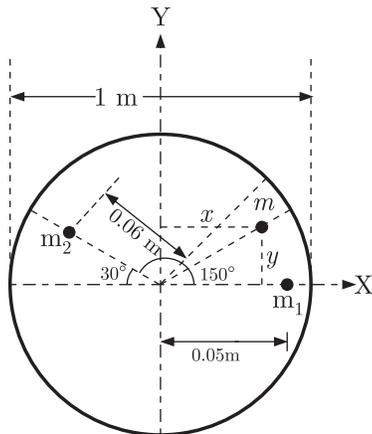
Given  $m_1 = m_2 = 0.5 \text{ kg}$ ,  $r_1 = 0.05 \text{ m}$ ,  $r_2 = 0.06 \text{ m}$
